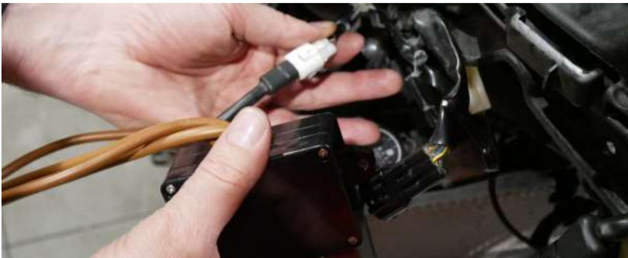
Fix the control unit to the frame of the bike in the area indicated in the figure by means of medium-sized plastic clamps. Do not worry about engine heat or vibration as the electronic box has been designed to withstand those working conditions without any problem and will not suffer any damage.
