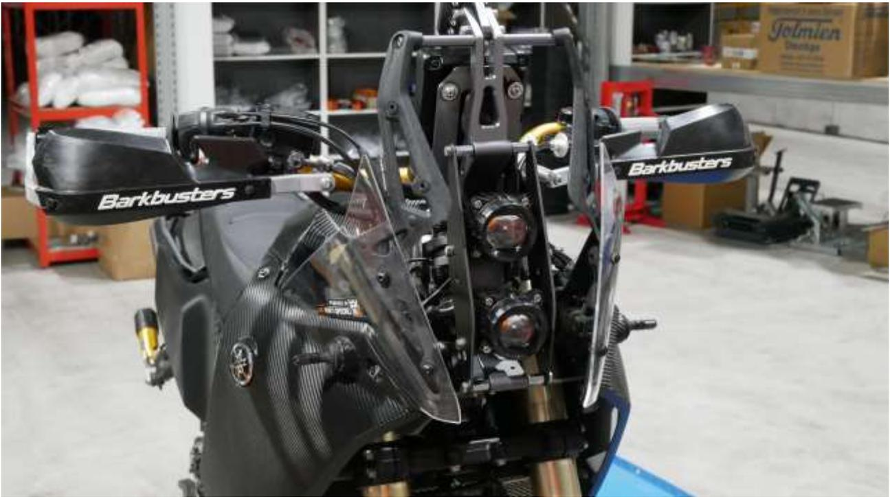
Then position the fairing aligning it with the original fairings.
