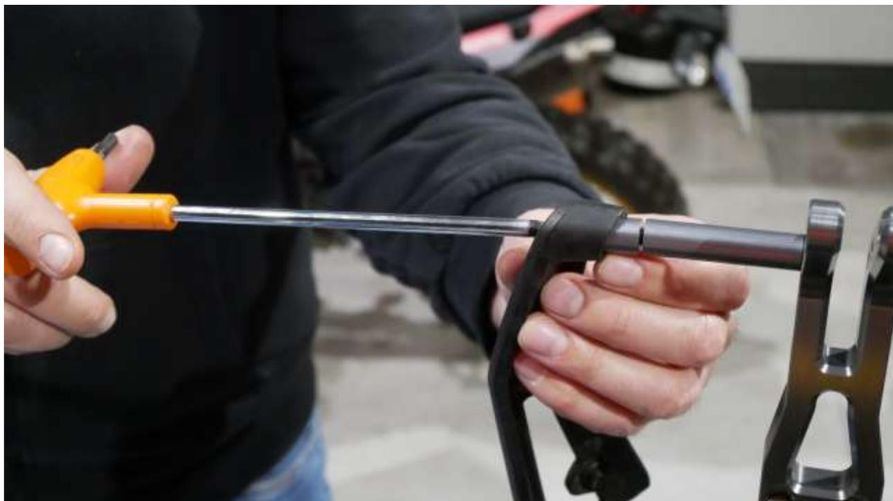
Now perform the fixing of the lower fairing support. It may be necessary a slight adaptation of the support bracket by sliding inside the slots. Once you have found the correct position, proceed to tighten the 2 screws using the self-locking nuts. Be careful, do not tighten excessively to avoid damage to plastics.
