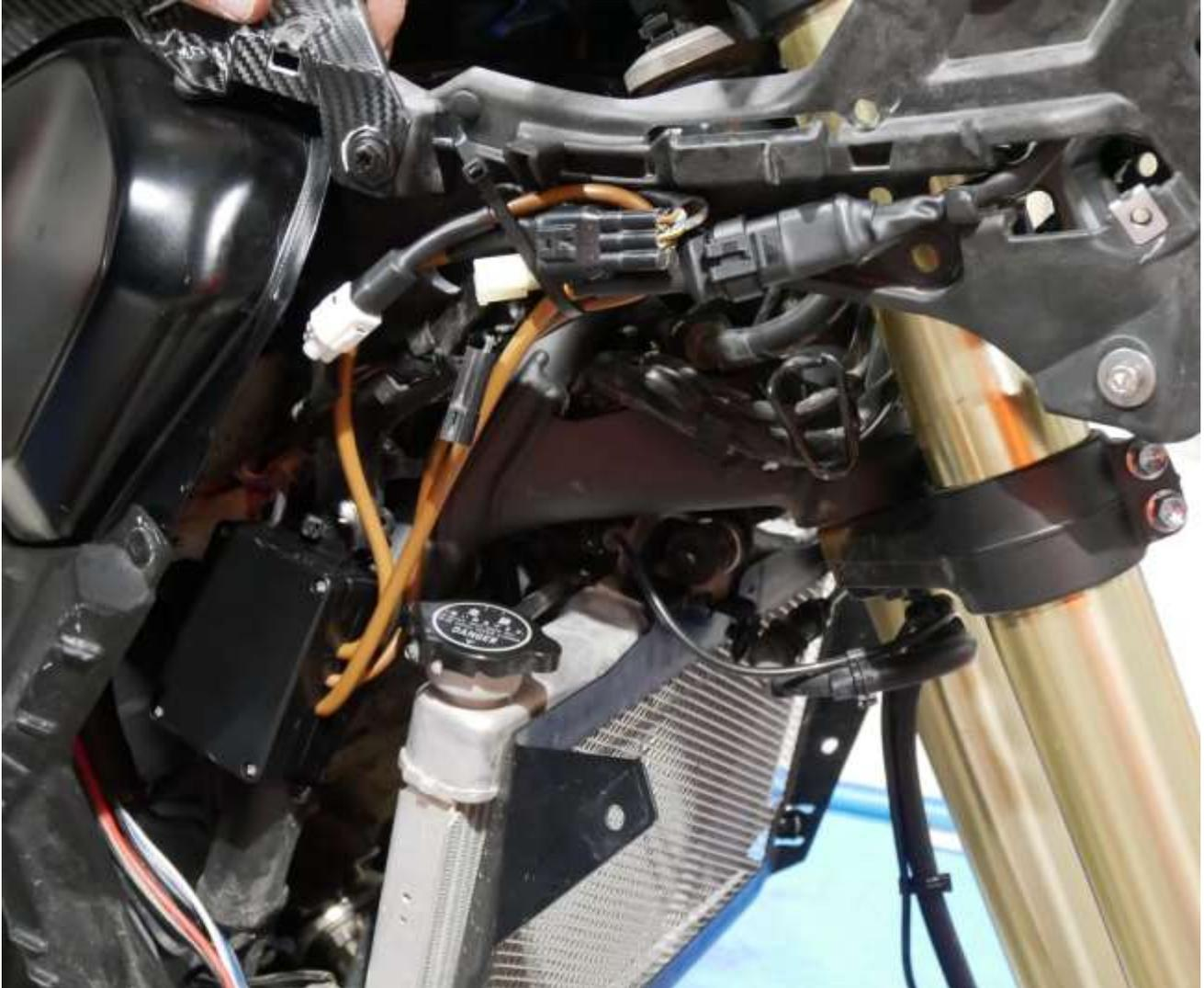
At this point you can turn on the panel of the bike and check that you have correctly connected the 2 headlight connectors (high beam headlight, low low beam headlight). If not, turn off the electrical panel and reverse the connectors.
