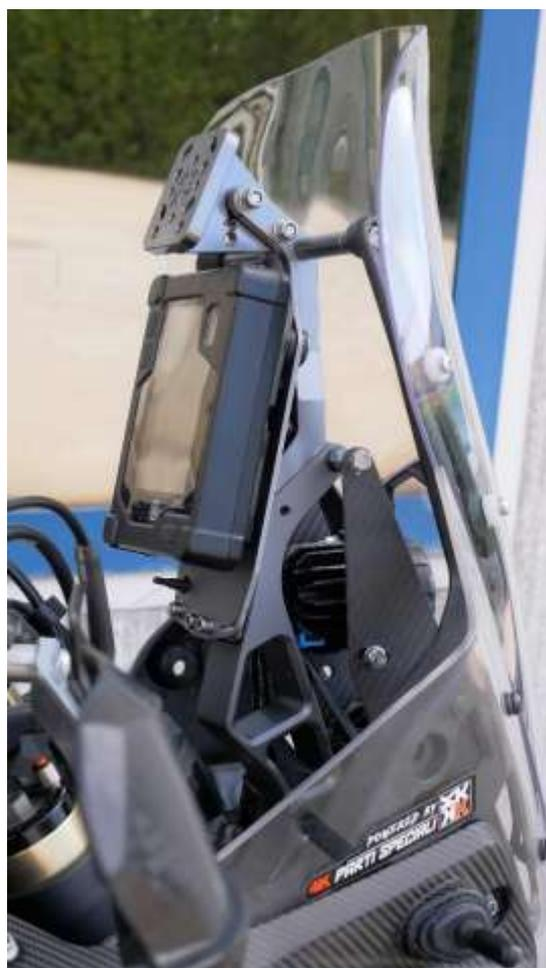
The first operation is to completely disassemble the original front end of the bike. It is a rather simple operation, if you find difficulties you can use the Yamaha workshop manual and follow the instructions for dismantling the headlight. Then remove the plastics, the original headlight and the headlight support. The result is the one in the picture below
