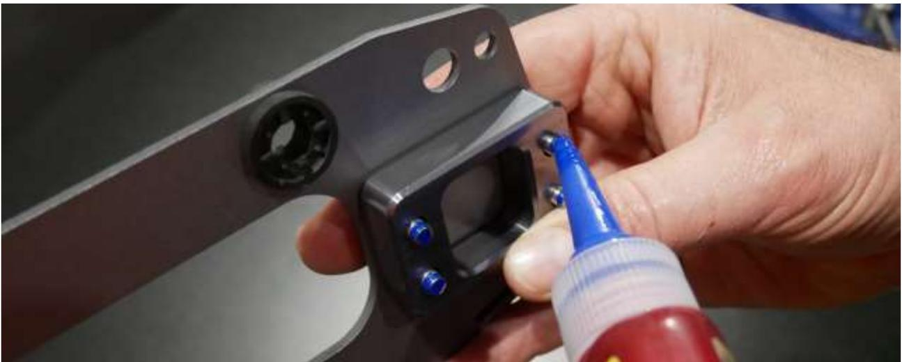
Fix the instrument support, taking care to first pass inside the original instrument connector of the bike (marked in red in the picture). Tighten the screws by hand, do not force.
