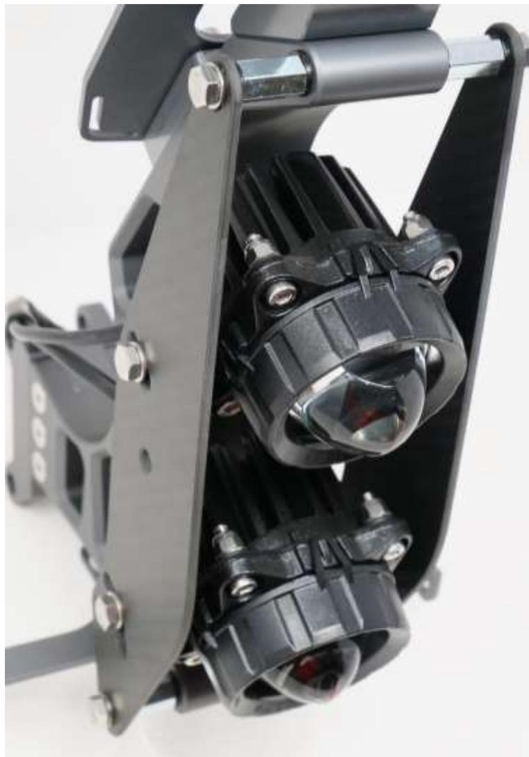
Prepare the bench instrumentation support, inserting the original instrument grommets into the new sheet metal by hand. In case of difficulty in insertion, use lubricant (e.g. WD-40). Then apply medium threadlocker to the M5 fixing screws
