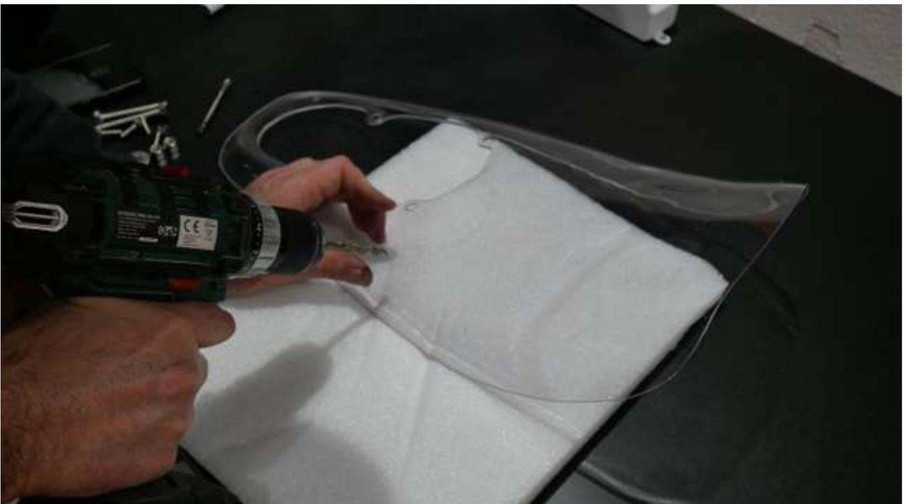
Screw the fairing using the spacers provided in the kit without exceeding by force to avoid cracks or damage to the polycarbonate.
