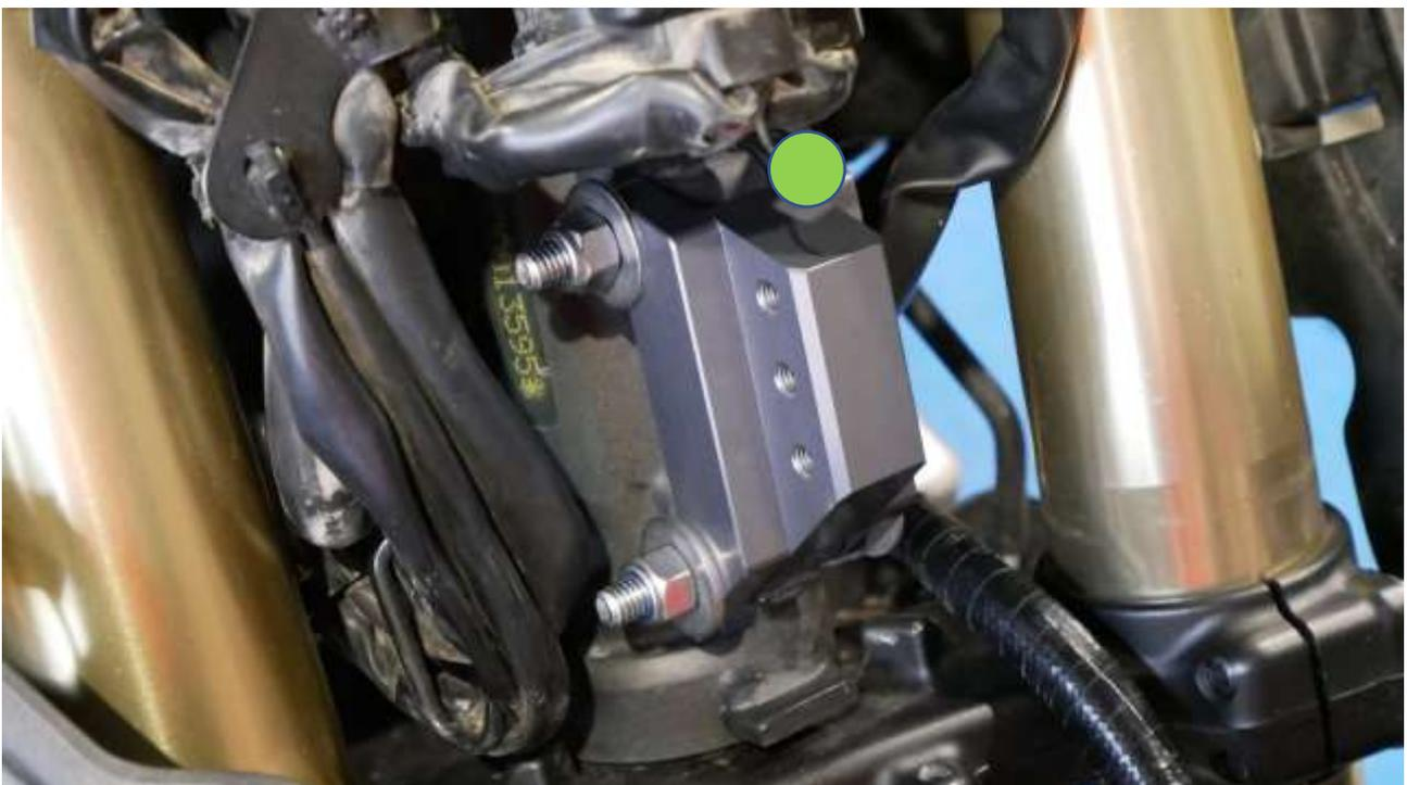
Tighten the screws tightly until the interface, due to deformation, no longer presents play on the frame of the bike
