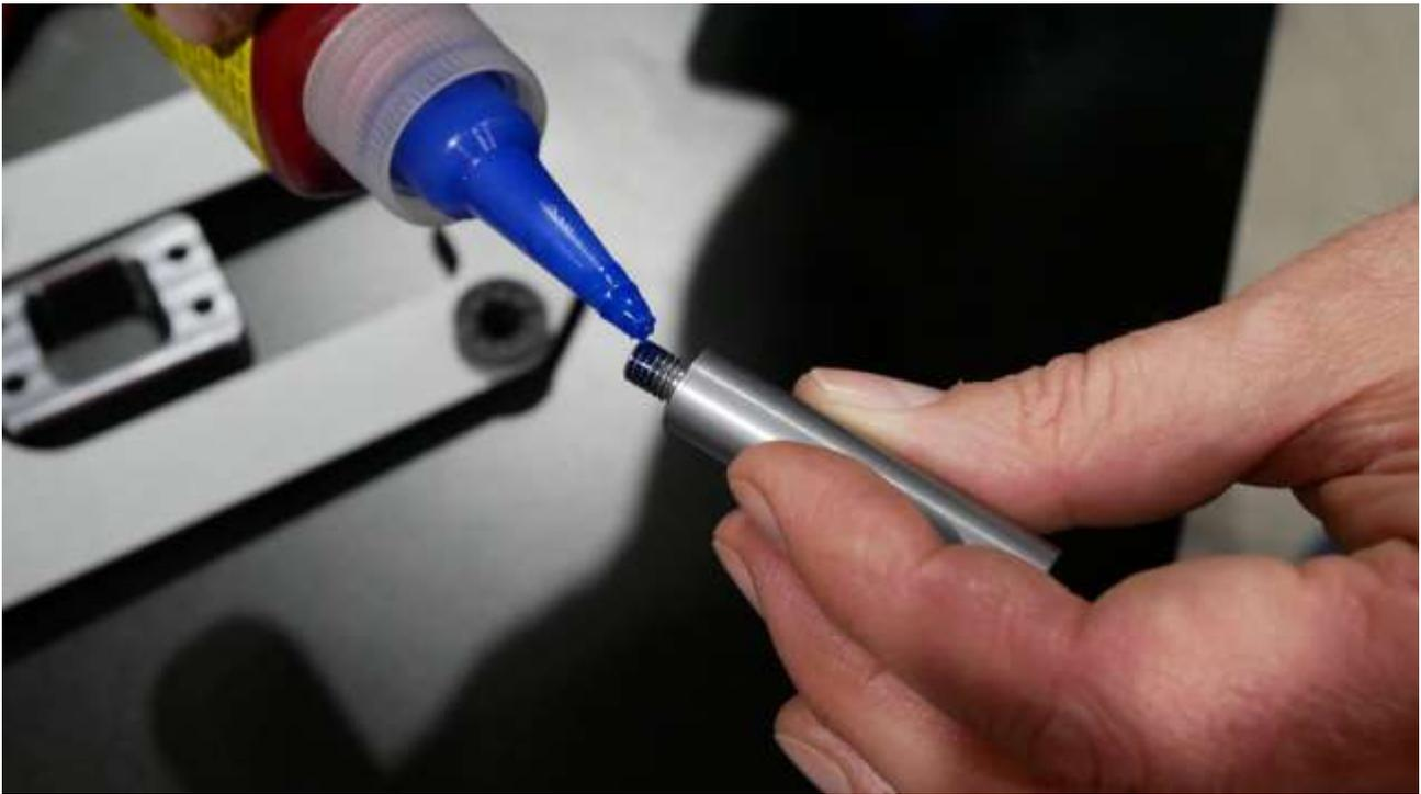
**Screw it firmly by hand to the stop, do not use pliers or other tools to tighten it!**
