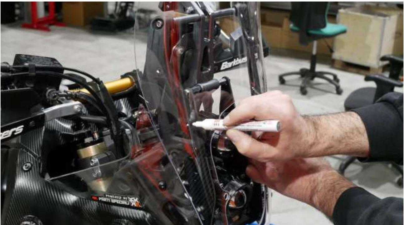
With a marker then accurately mark the location of the holes. Bring the fairing to the bench and drill with a drill (we recommend 6mm holes, if necessary enlarge).
