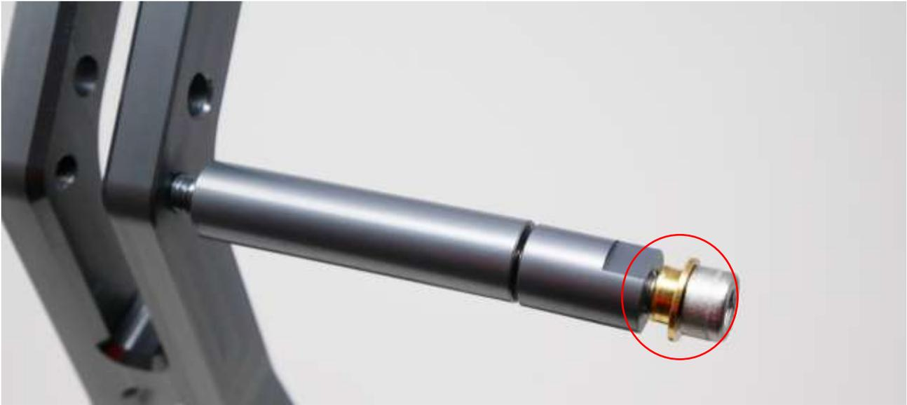
Then apply medium threadlocker to the first threaded cylinder
