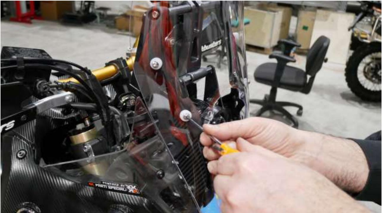
Insert the 4 nuts with rubber flange in the kit (part threaded inwards) into the headlight window.
