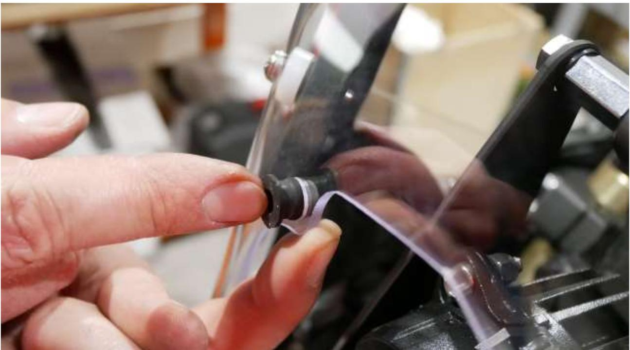
Then apply the headlight cover and the anti-reflective insert.
