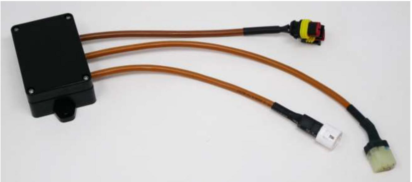
On the right side of the bike you will find the few cables that come from the original electrical system. We have restored the same connectors so as to leave no possibility of error and allow a quick assembly with a click.
