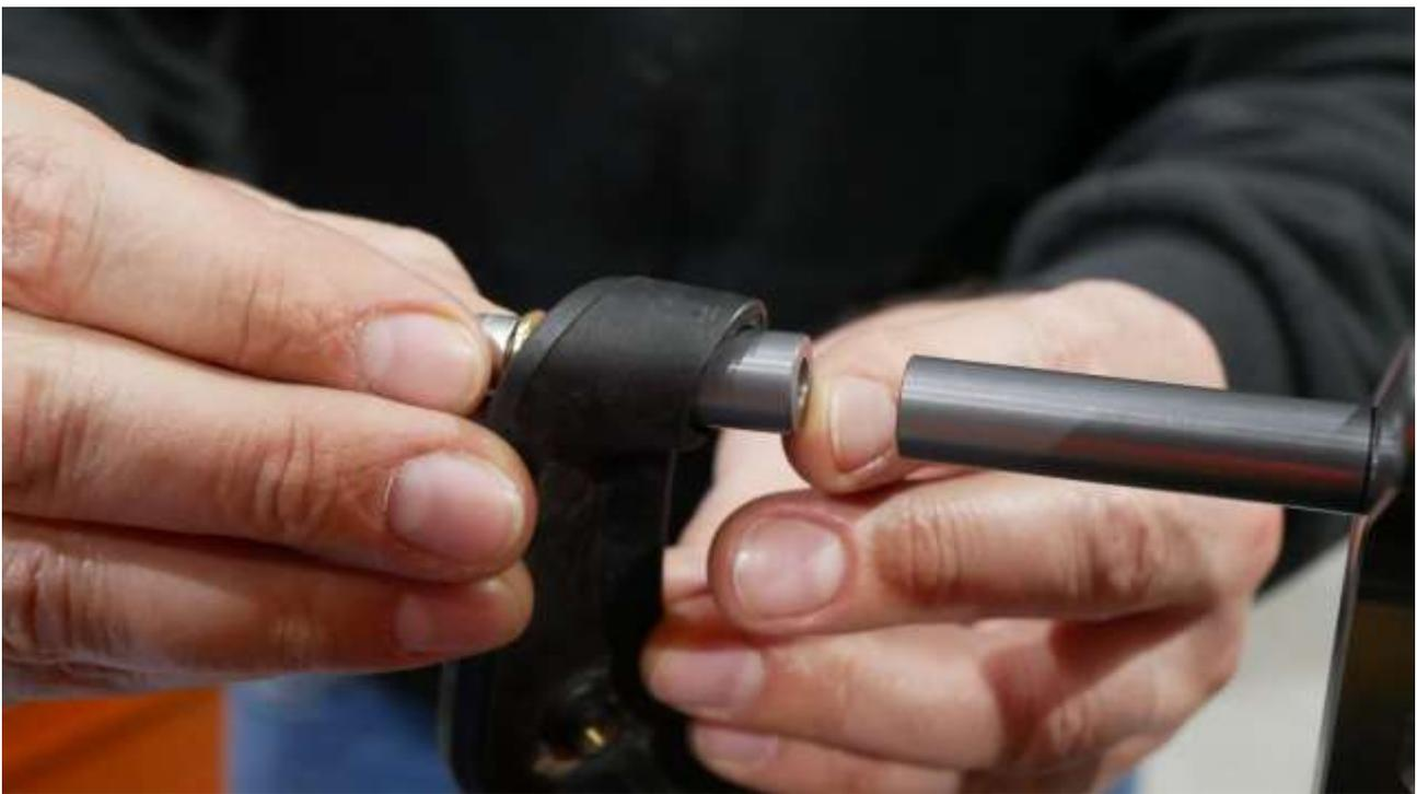
Tighten everything with a key. It is not necessary to apply excessive force. Once you have done so, repeat for the other side. Now the composite fairing of the bike are supported by the turret through the upper part.
