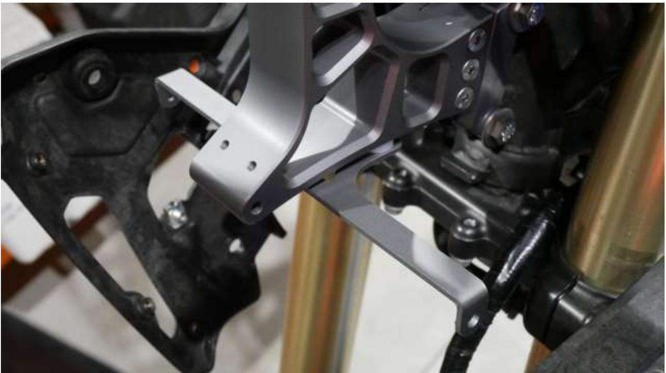
We proceed to the assembly of the instrumentation support in the upper part of the turret.
