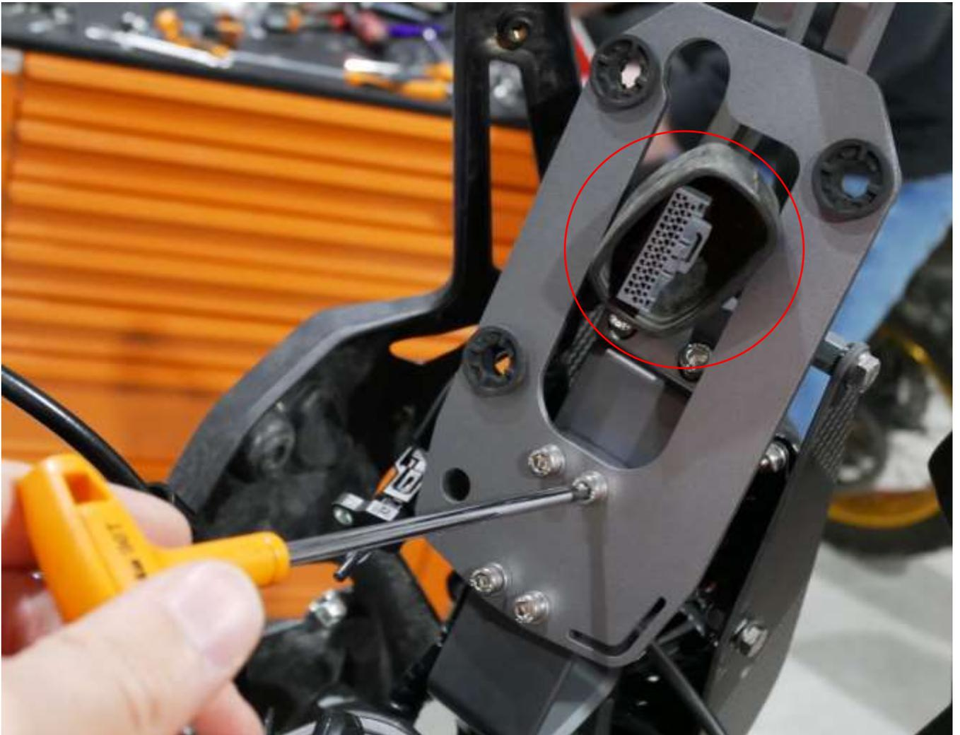
With an M6 screw and self-locking nut, proceed to fix the temperature sensor in the appropriate hole of the instrument plate as shown in the picture
